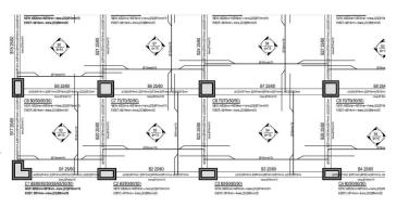
Finally, the technical report of the analysis can be created on-the-fly in PDF, RTF or HTML file formats, whereas a variety of CAD drawing files of the building structural model (plan views, cross sections and reinforcement tables) may be quickly created and exported.
