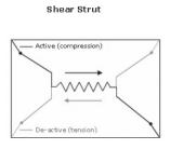
corners and a third one to carry the shear from the top to the bottom of the panel. This latter strut only acts across the diagonal that is on compression, hence its "activation" depends on the deformation of the panel. The axial load struts use the masonry strut hysteresis model, while the shear strut uses a dedicated bilinear hysteresis rule.
