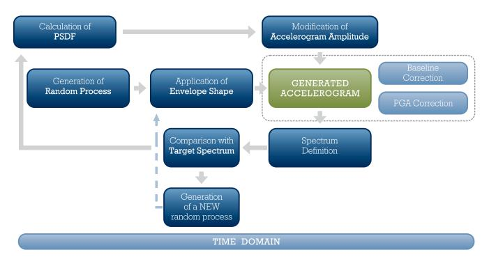
The software automatically carries on the entire iterative procedure. N executions with different ( $N_{\omega}$ ) phase angles are performed until convergence is reached. The default values are N=3 and  $N_{\omega}$ =100 as can be noted in the Program Settings module of the software. If convergence cannot be reached, SeismoArtif will output the best solution.
