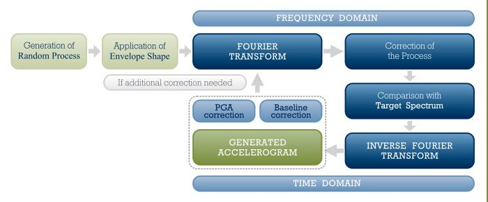
Input parameters and output results are the same of the Artificial Accelerogram Generation method, but this is more stable and one-sided and more likely to lead to a very good convergence (error less than 7-8%), at the expense of a higher number of iterations, however.
