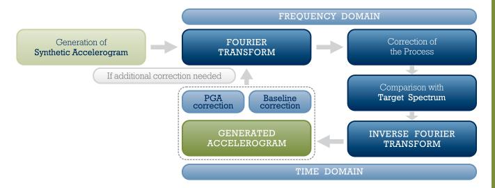
In this calculation method framework, the Envelope Shape module is not required, since the procedure does not start from a random process, but rather from a synthetic accelerogram.
