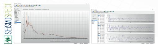
SeismoSpect allows users to open accelerograms from text files in different formats, to create their own library of ground motion records and save them all in a single file making it easy to handle and share large numbers of records. It features a user-friendly visual interface and is capable of deriving a number of strong-motion parameters often required by engineer seismologists and earthquake engineers.
