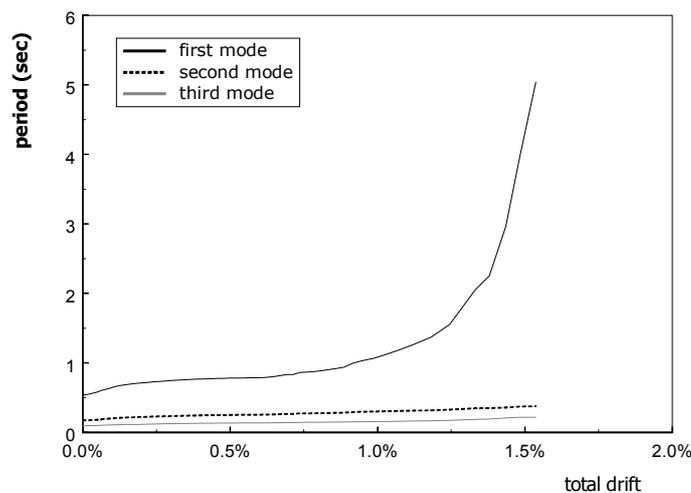
Figure 3. Periods of vibration of 4-storey building under increasing levels of deformation.
