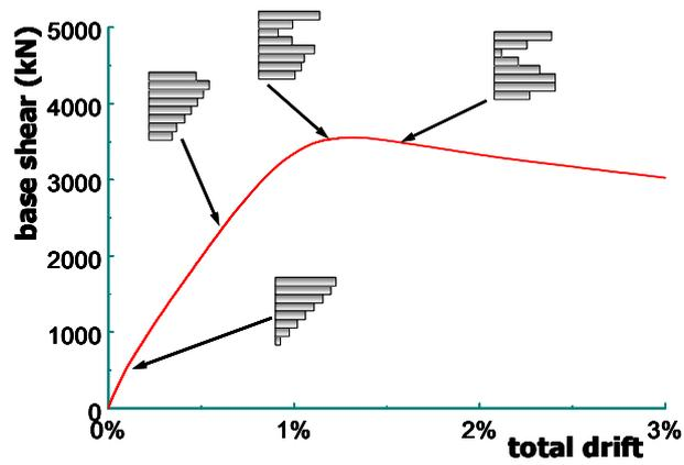
Figure 5. Adaptive pushover: shape of loading vector is updated at each analysis step.
