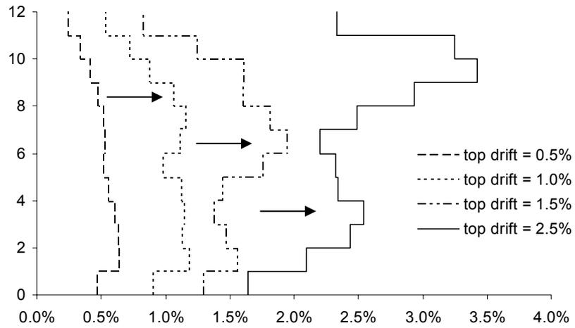
Figure 4. Interstorey drift profiles of a 12-storey building subjected to increasing levels of deformation.
