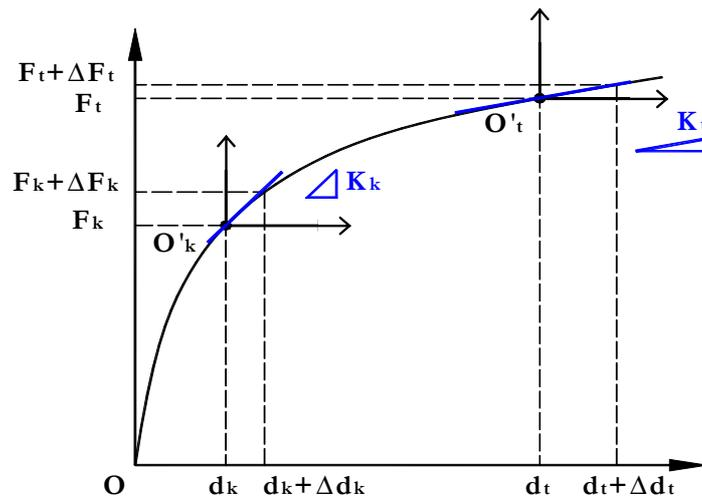
Figure 6. The use of tangent stiffness in updating (i.e. incrementing) the loading vector.
