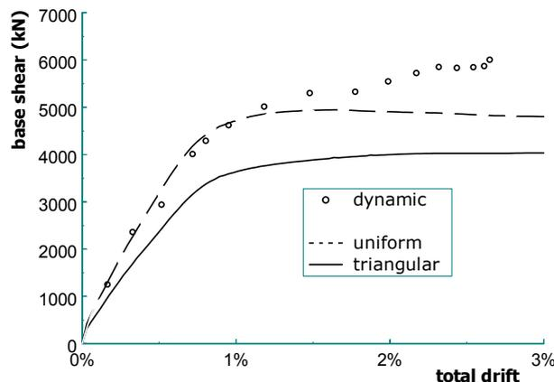
Figure 1. Capacity curves of a 12-storey building, obtained with standard pushover and Incremental Dynamic Analysis
