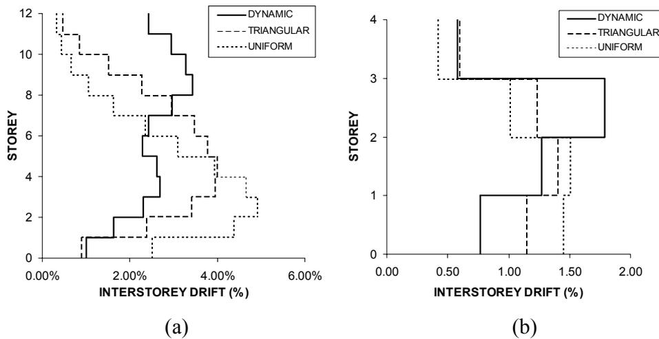
Figure 2. Interstorey drift profiles of (a) 12-storey building and (b) 4-storey irregular frame, obtained with standard pushover.
