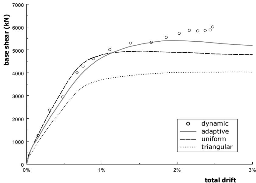
Figure 8. Capacity curves of a 12-storey building, obtained with DAP and standard pushovers, and compared against IDA envelopes.
