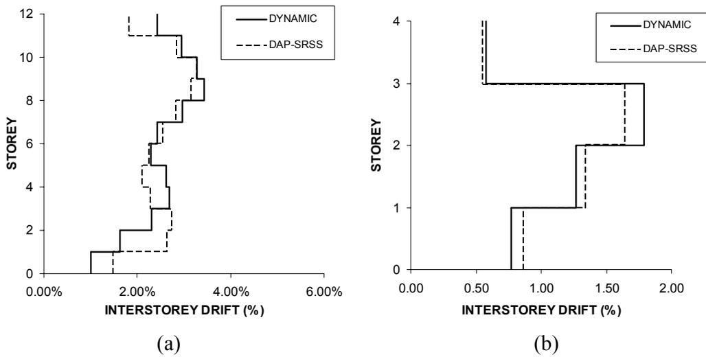
Figure 7. Interstorey drift profiles of (a) 12-storey building and (b) 4-storey irregular frame, obtained with Displacement-based Adaptive Pushover using SRSS combination.
